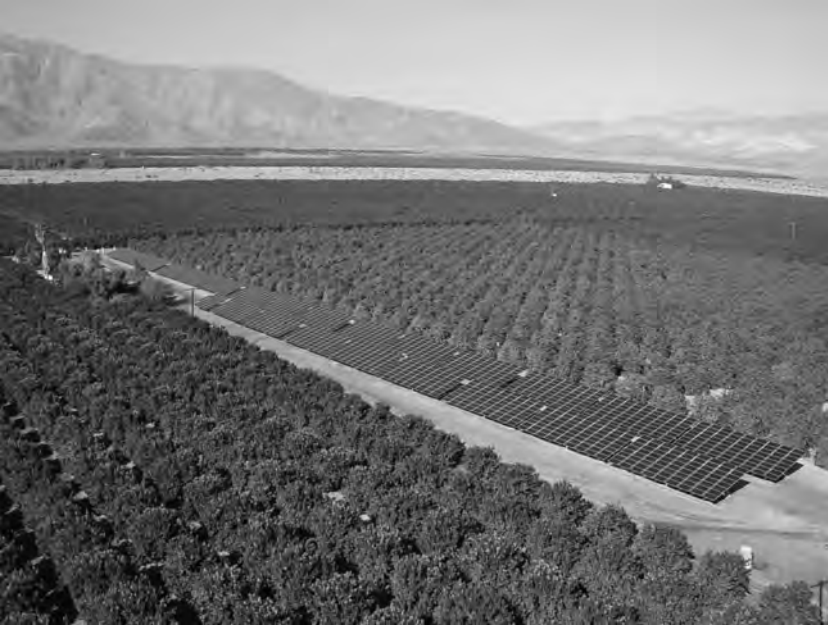
Figure B.19 Solar power cogeneration for agricultural water irrigation. Photo courtesy of WaterWorld.
