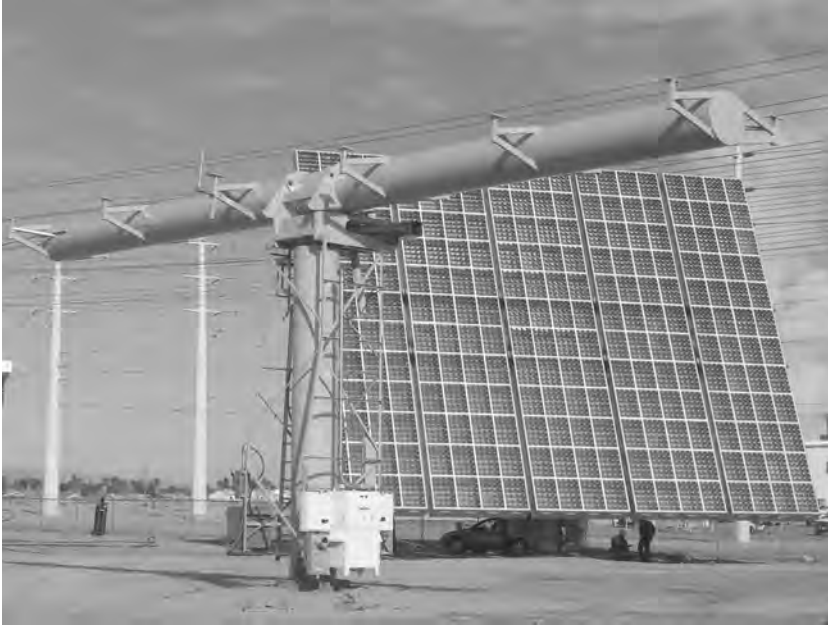
Figure 2.10 MegaConcentrator module two axis hydraulic tracking system. Photo courtesy of Amonix.
