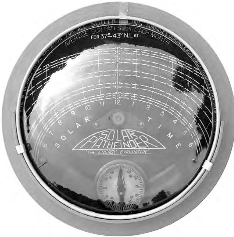
Figure 4.7 Spherical dome showing the reflection of surrounding buildings and vegetation. Photo courtesy of Solar Pathfinder.
