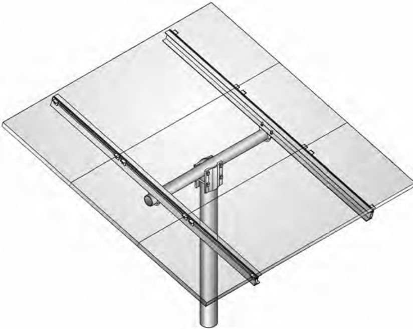
Figure B.13 Roof-mount fixed tilt PV support system using simple channel hardware.
