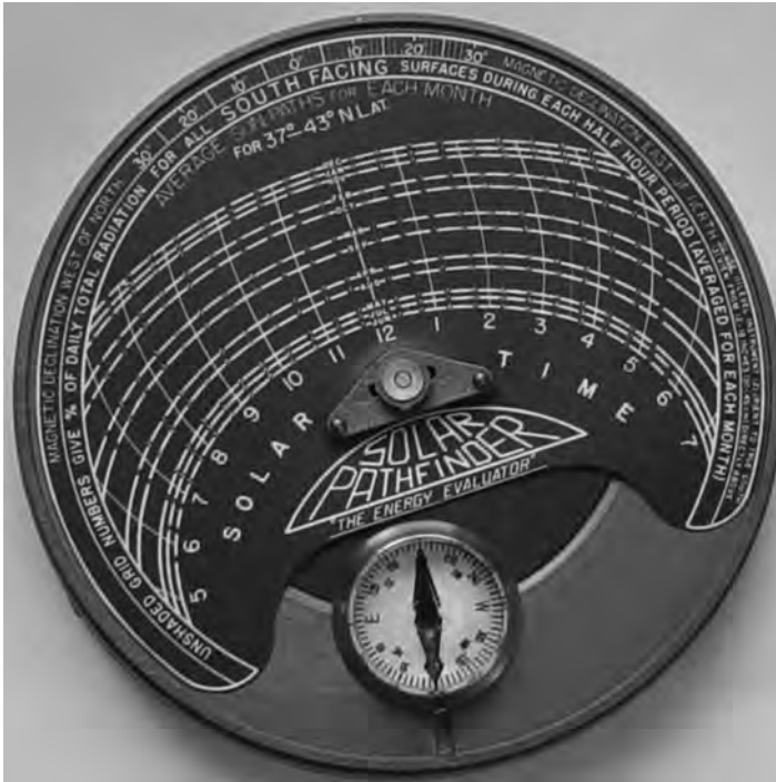
Figure 4.10 The Solar Pathfinder showing the removable shading graph, the leveling bubble at the center and the compass. Photo courtesy of Solar Pathfinder.
